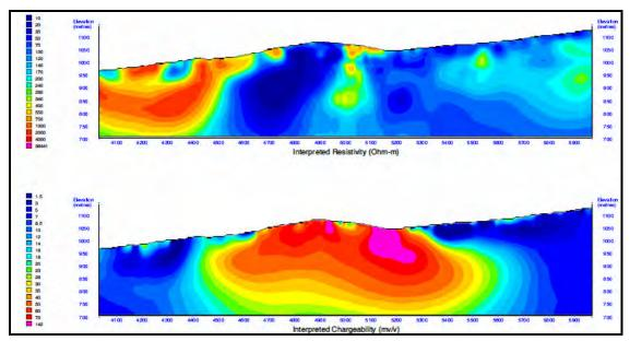
Figure 10.4 Line 4800- 3D Cross Section – Interpreted Resistivity and Chargeability
