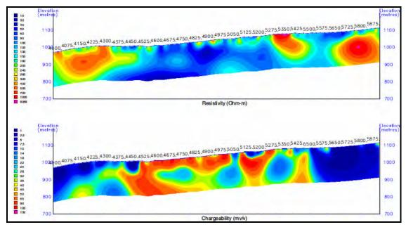
Figure 10.8 Line 4200n Interpreted Resistivity and Chargeability
