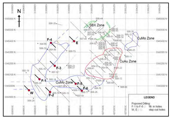
Figure 17.1 Proposed Drilling
