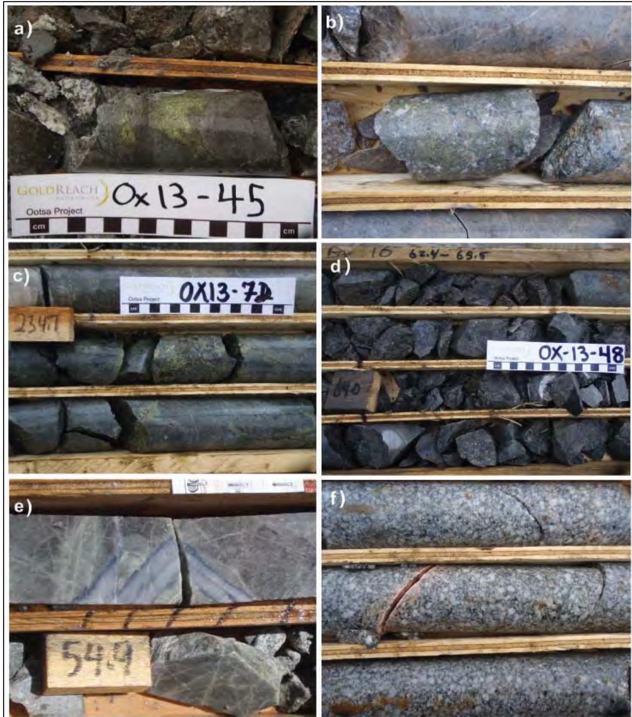
Figure 7-12: Photographs of drill core from the Ox deposit: a) brecciated sedimentary rock with strong chalcopyrite mineralization and late white calcite veins; b) altered fine-grained feldspar porphyry sill with sulfide mineralization; c) chalcopyrite and pyrite in dark biotite hornfels sedimentary rock; d) rubbly mineralized zone with inferred anhydrite dissolution; e) quartz vein with grey molybdenite in the vein centre and along the vein selvages; and f) coarse, crowded feldspar-biotite porphyry intrusion that occurs on the east side of the Ox deposit (note the pink K-feldspar vein in the middle row)
